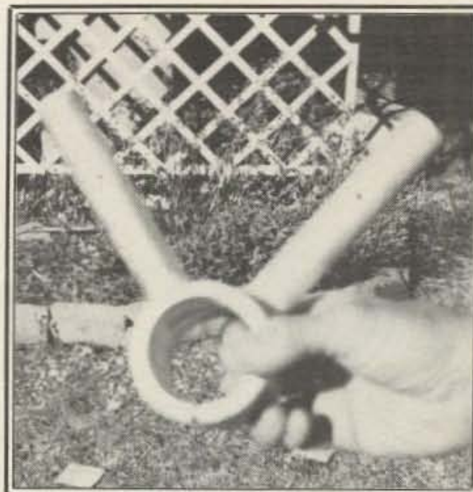
Here is one of the element supports.
